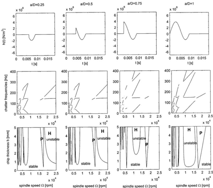
Figure 2. Down-milling, number of cutting teeth  $N = 1$ , specific cutting force variation diagrams, frequency diagrams and stability diagrams for varying immersion ratios  $a/D=0.25, 0.5, 0.75, 1$
