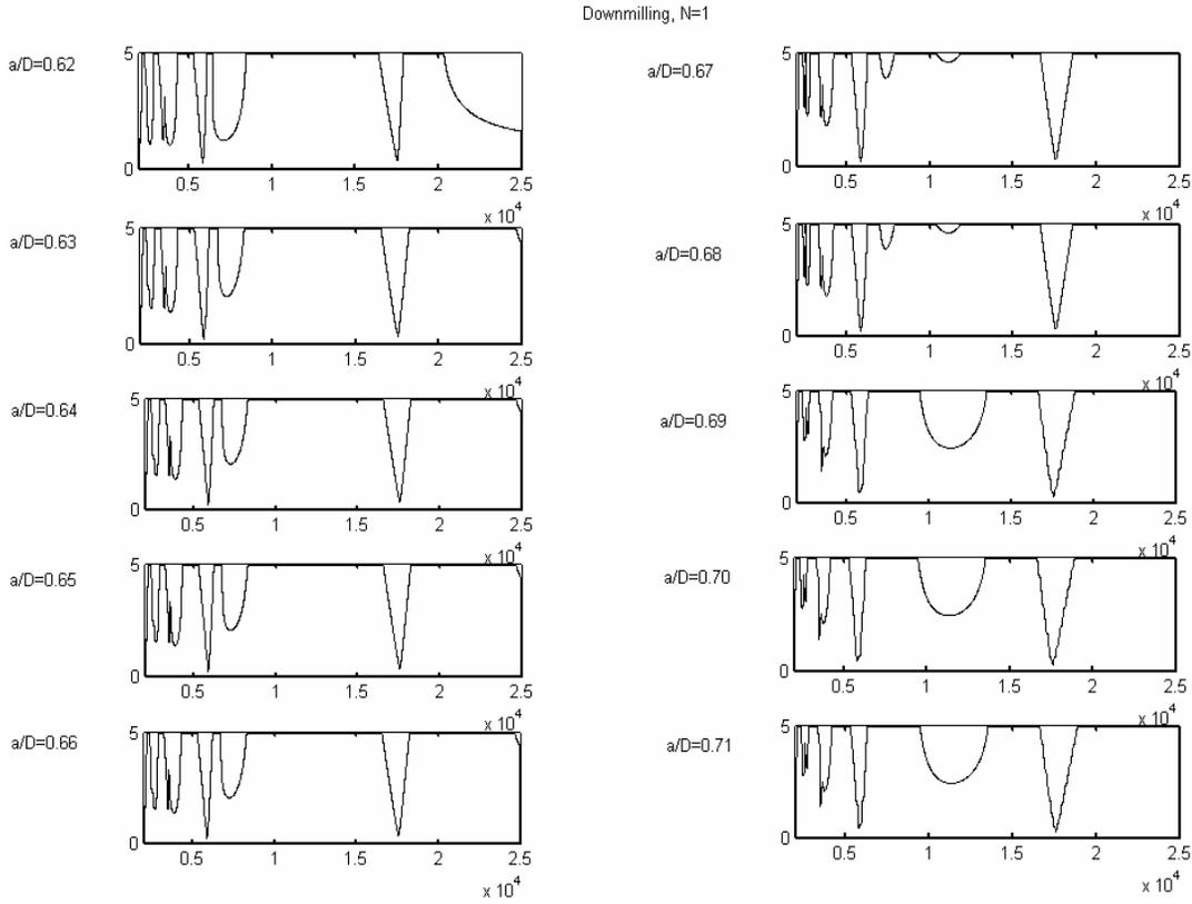
Figure 7. Critical immersion ratios for down-milling,  $N = 1$ , collocation points  $m = 80$ , parameter plane  $300 \times 300$  grid points
