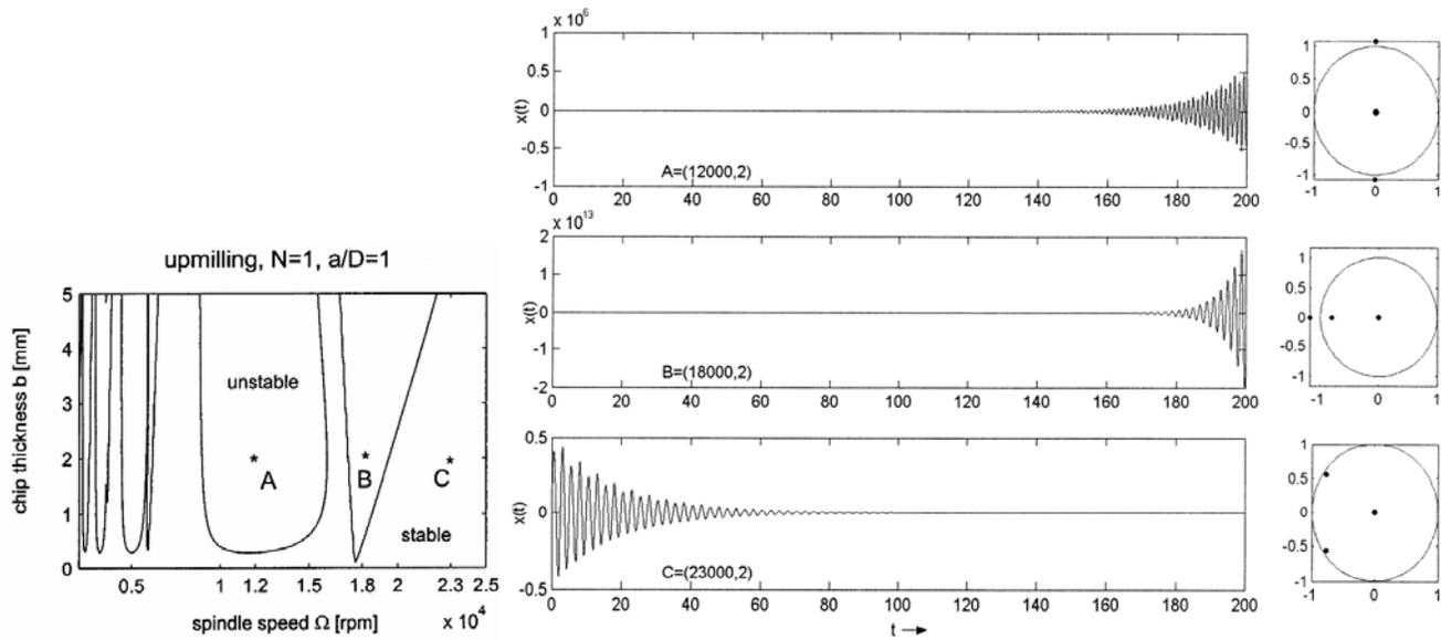
Figure 5. DDE23 results for the parameter points A, B and C picked from the stability diagram of up-milling with  $N = 1$ ,  $a/D = 1$  and collocation results for finding the locations of characteristic multipliers
