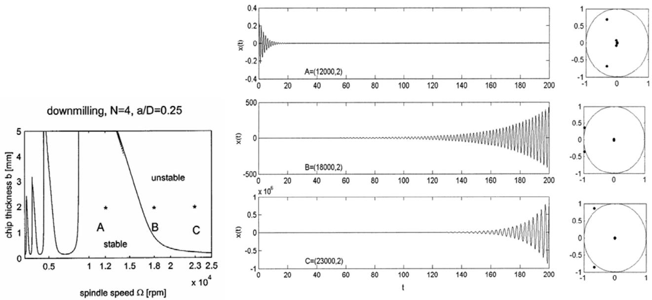
Figure 6. DDE23 results for the parameter points A, B and C picked from the stability diagram of down-milling with  $N = 4$ ,  $a/D = 0.25$  and collocation results for finding the locations of characteristic multipliers
