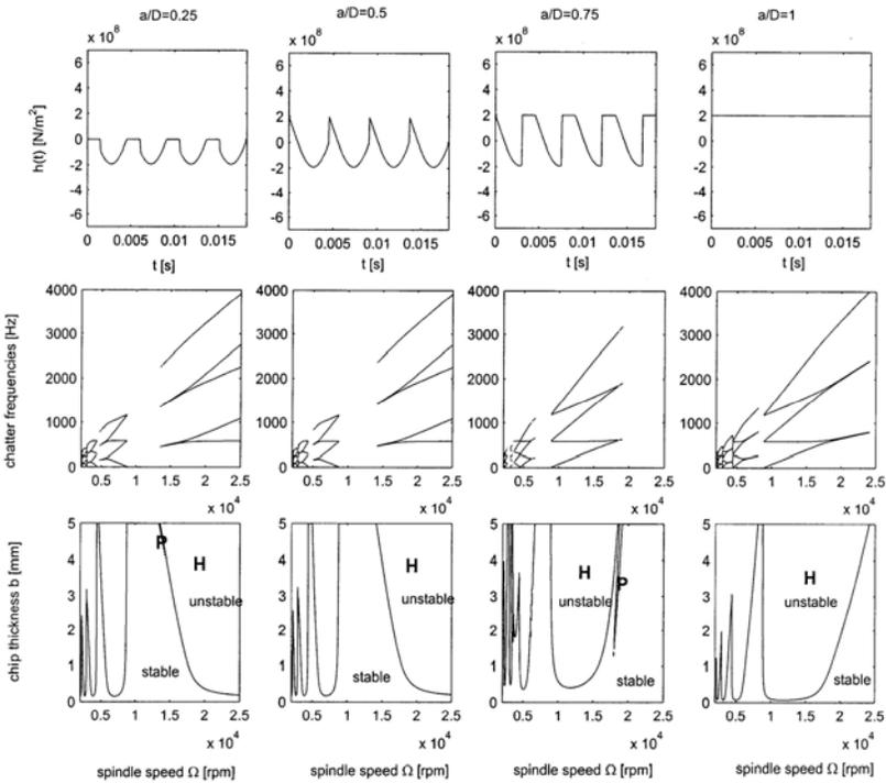
Figure 4. Down-milling, number of cutting teeth  $N = 4$ , specific cutting force variation diagrams, frequency diagrams and stability diagrams for varying immersion ratios  $a/D=0.25, 0.5, 0.75, 1$
