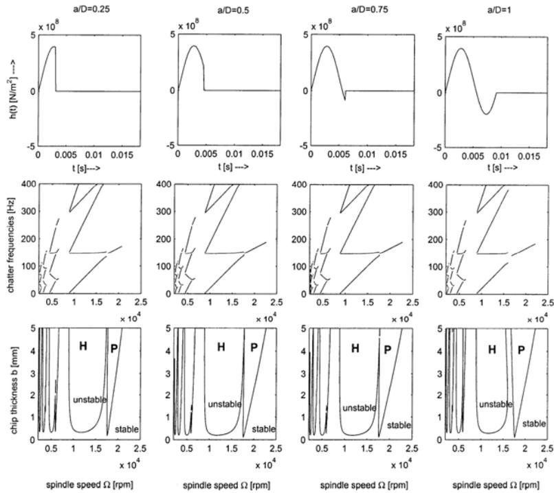
Figure 1. Up-milling, number of cutting teeth  $N = 1$ , specific cutting force variation diagrams, frequency diagrams and stability diagrams for varying immersion ratios  $a/D=0.25, 0.5, 0.75, 1$
