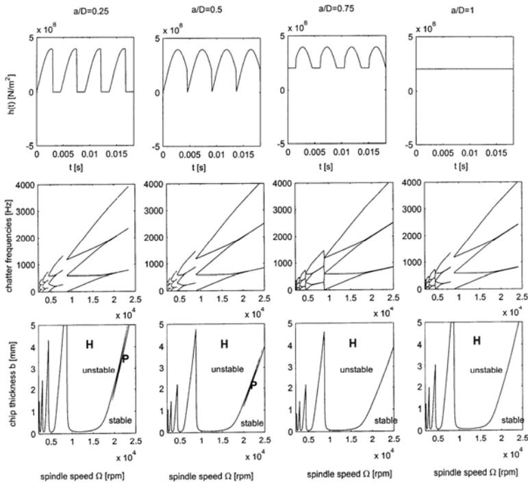
Figure 3. Up-milling, number of cutting teeth  $N = 4$ , specific cutting force variation diagrams, frequency diagrams and stability diagrams for varying immersion ratios  $a/D=0.25, 0.5, 0.75, 1$
