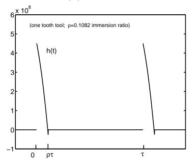
QUESTION: Suppose m, c, k fixed. For which values of parameters  $\Omega = 60/\tau$  and w is this milling DDE stable?
