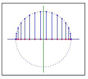
Note  $t_j \in [-1, 1]$ . If needed, shift and scale the collocation points to interval  $[0, \tau]$ .
