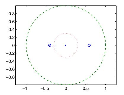
*Proposition* (with *a posteriori* proof): If  $\mu$  is an eig of U and  $|\mu| \ge 0.3$  then  $\mu$  is in one of the discs.
